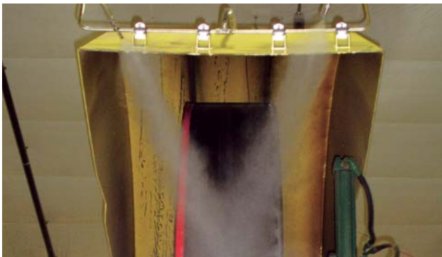
1-2 nozzles are mounted on top of the machine to knock down the fine dust that comes out of the hood.
