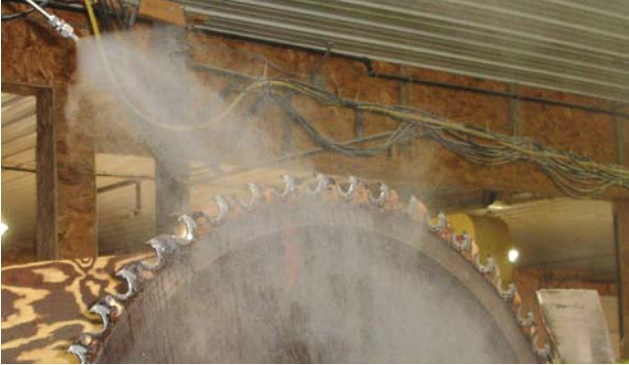
One nozzle sprays directly on the saw blade to clean and cool the saw. Additional nozzles can be installed to knock down dust in the air around the saw.
