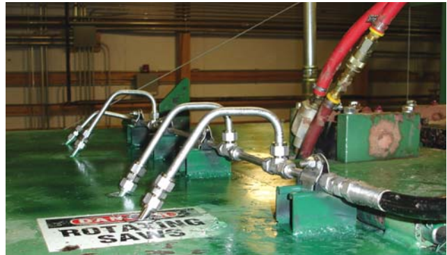
2-5 small nozzles are mounted inside the machine and spray directly on the saws to clean and cool them.
