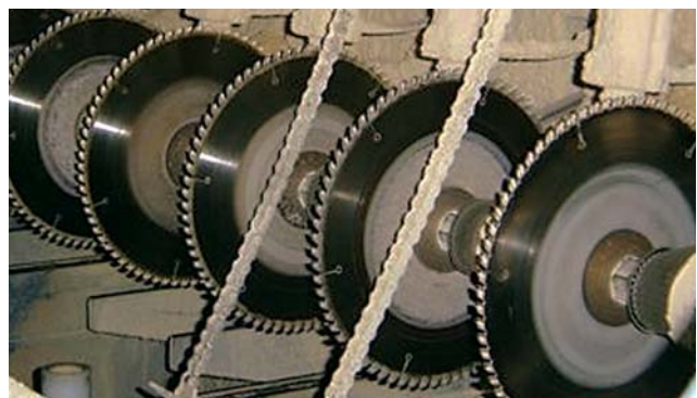
Several nozzles are mounted inside the trimmer and they spray directly on the saws to clean and cool them.
