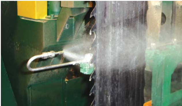
One nozzle sprays directly on the saw blade to clean and cool the saw.
