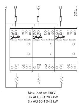
Three phase with single-phase contactor ECI-1 as slave Only burst firing mode
