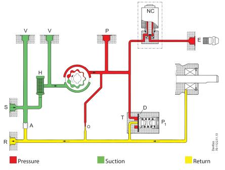
From the suction inlet (S) oil is drawn through the filter (H) to the gear set, where the pressure is increased. When voltage is applied to the NC-valve, it opens and releases oil to the nozzle outlet.
