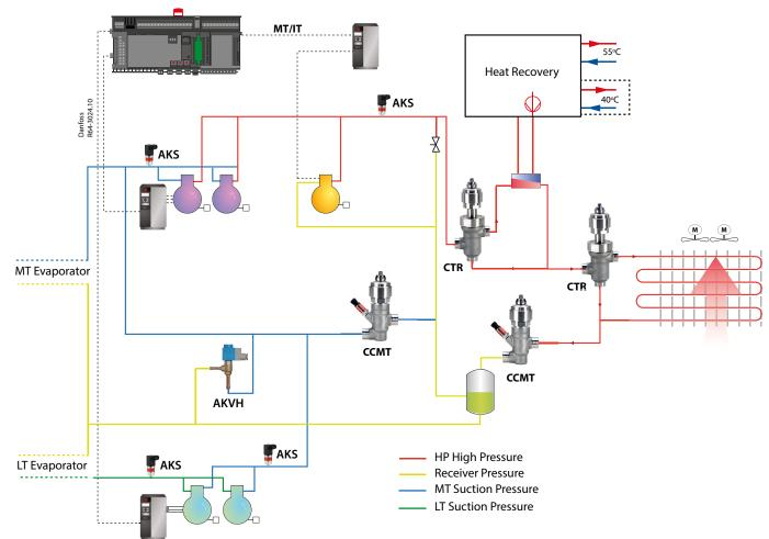
In  $CO_2$  systems, the higher pressure and temperature make it possible to recover heat for tap water and heating. The excess heat is removed using a gas cooler.
