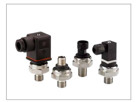
The P500 utilizes the thin film strain gauge sensing technology, incorporating an hermetically sealed design with no internal sealing required. Designed for harsh environments, a rugged 304 stainless steel housing surrounds the P500 transducer.
