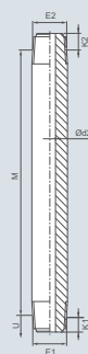
Neck tube, nipple, non adjustable, conical, european (4), american (6), dimensions in mm (inch)
