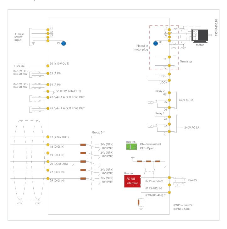
The diagram shows the terminals of the VLT® DriveMotor FCM 106 and VLT® DriveMotor FCP 106.
