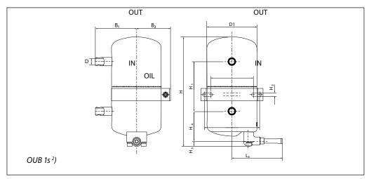
$^{2}\hspace{-0.5mm}$  ) 6 mm ODF solder connection to oil return line.
