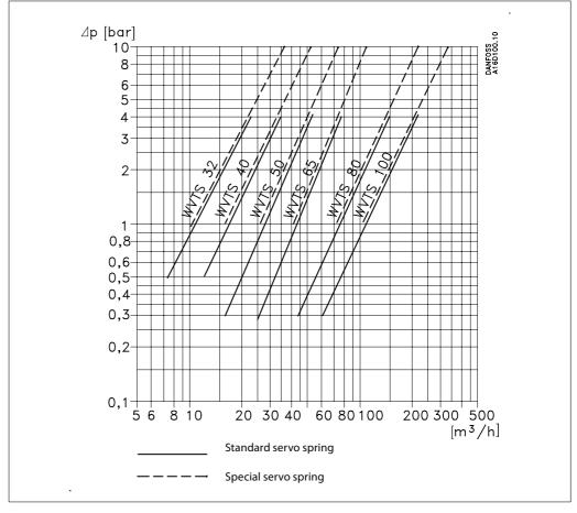
The capacity curves show the capacity (water quantity in [m³/h]) of the individual valve sizes as a function of pressure drop across the valve.
